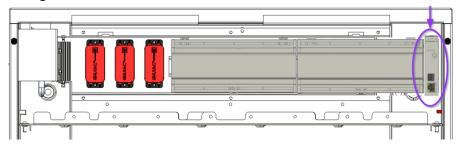
8. Connect the RMG/941C cable to the Hyperion board and the RJ45 Cable to the pass-thru socket.
